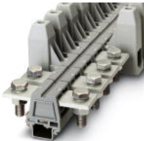
Universal terminal block with bolt connection, cross section: 50 ... 150 mm 2 , width: 46 mm, color: gray
