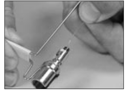
3.12 Gently insert the fiber into the connector.
