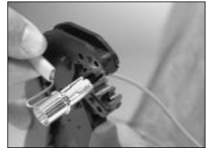
6.21 Crimp the larger part of the crimp ring with the .190 cavity of the crimp tool.
