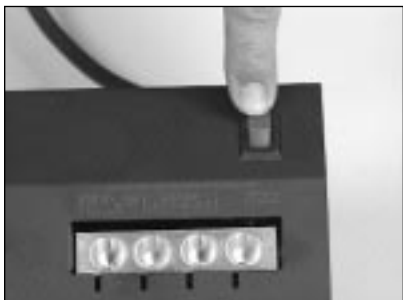
6.1 Turn on the Hot Melt oven. The oven requires 5 minutes to warm up.
