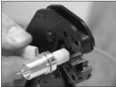
8.20 Crimp the larger part of the crimp ring with the .190 cavity of the crimp tool.
