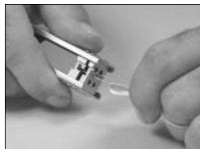
6.12 Remove the buffer in small pieces until 1/16"–5/8" (14-16 mm) of the buffer remains.
