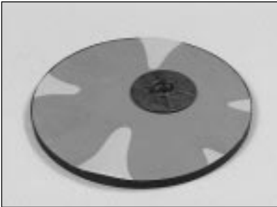
11.10 Place the jig on the lapping film.
