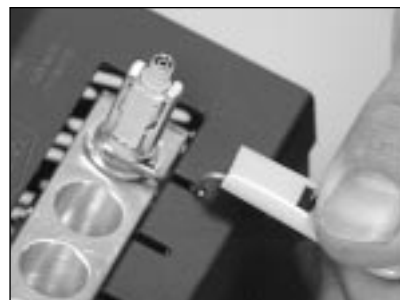
6.6 Place the connector holder and connector into the oven.
