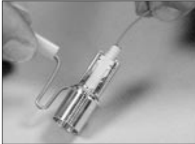
5.13 Push the buffered fiber until it stops.
