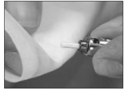
11.24 Clean the connector end face with a lint free cloth moistened with isopropyl alcohol.
