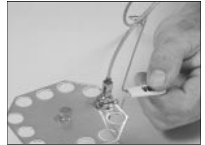
4.21 Place the connector holder into the cooling stand. The cooling time is about 3 minutes.
