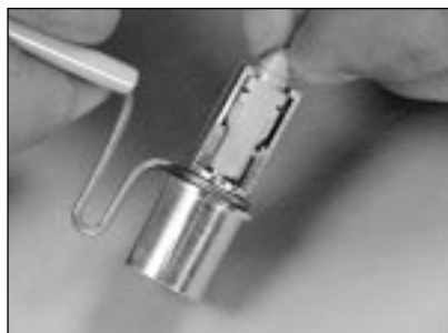
6.5 Push down on the connector and turn it 90 degrees so that the arms hold the connector in place.
