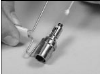
4.17 Gently insert the fiber into the connector.
