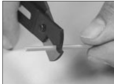
4.8 Score the jacket \frac{3}{4} " (19 mm) to \frac{7}{8} " (22 mm) from the end.
