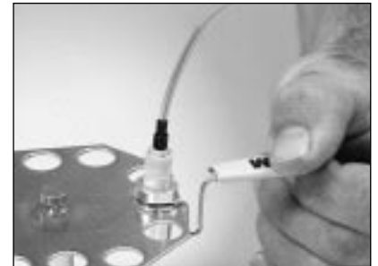
7.18 Place the connector holder into the cooling stand. The cooling time is about 3 minutes.
