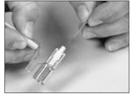
5.12 Gently insert the fiber into the connector.
