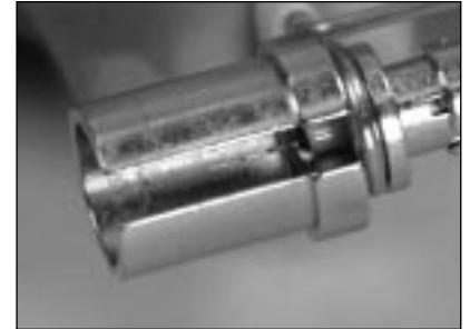
3.15 Bare fiber should be visible in the bottom of the connector holder.
