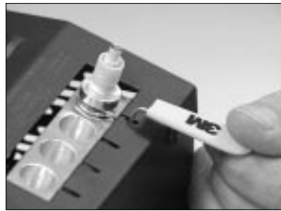
7.5 Place the connector holder and connector into the oven.
