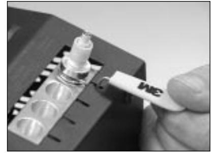
8.15 Remove the connector holder from the oven.
