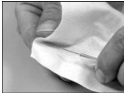
6.14 Clean the fiber with a lint free cloth moistened with isopropyl alcohol.
