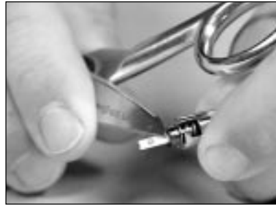
11.8 If the ferrule does not fit properly, there are two possible causes. The first is that there is adhesive on the ferrule. To remove the adhesive, use the scissors and gently scrape away the adhesive.
