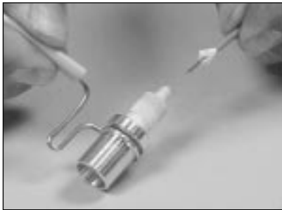
8.16 Gently insert the fiber into the connector.
