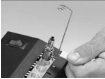
4.16 Remove the connector holder from the oven.
