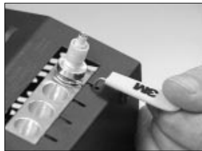
8.5 Place the connector holder and connector into the oven.
