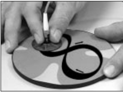
10.10 Place the jig on the lapping film.
