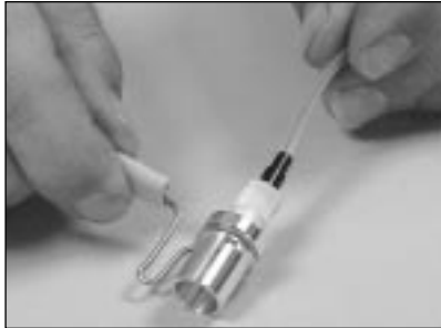
7.14 Slide the clear strain relief tube into the crimp ring.
