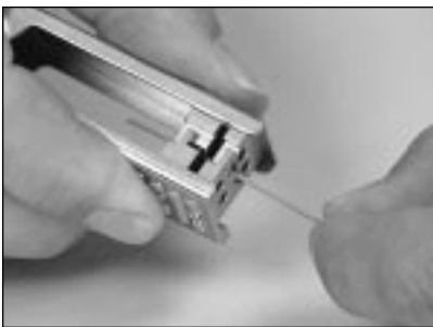
7.7 Remove the buffer in small pieces until \frac{9}{16} "– \frac{5}{8} " (14-16 mm) of buffer has been stripped.
