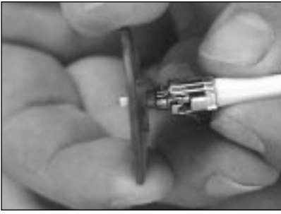
11.7 Place the connector ferrule in the polishing jig to verify that it fits properly. The fit should allow for easy movement of the ferrule.
