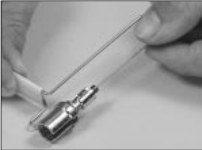
3.13 Push the buffered fiber until it stops.
