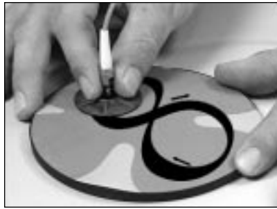
11.23 Polish the connector for 3 figure eights only.
