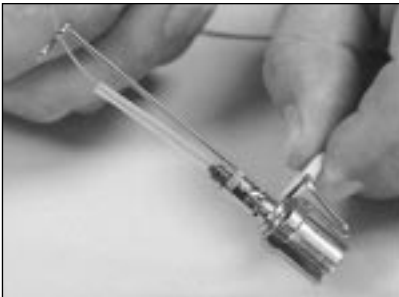
3.16 Place the buffered fiber in the cable holder.
