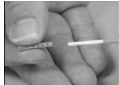
4.9 Remove the jacket from the end of the cable.
