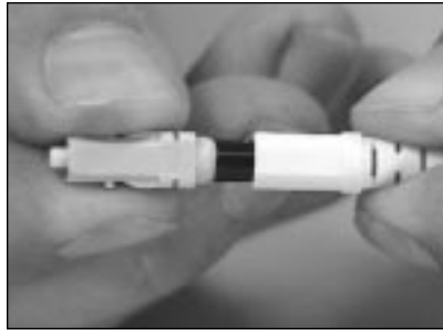
10.24 SC connector—Align the flats of the boot with the flat sides of the connector body.
