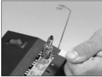
3.11 Remove the connector holder from the oven.
