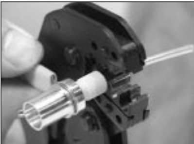
7.16 Crimp the larger part of the crimp ring with the .190 cavity of the crimp tool.
