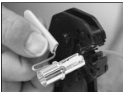
6.22 Crimp the smaller part of the crimp ring using the .137 cavity. (Use the .120 cavity for the optional 2.4 mm crimp ring.)
