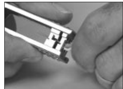
4.12 Remove \frac{5}{8} " (16 mm) of the buffer.
