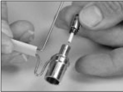
4.4 Load the connector onto the ST* connector holder.
