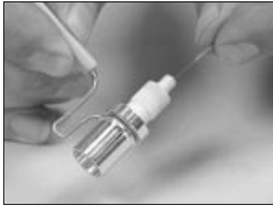
7.11 Gently insert the fiber into the connector.
