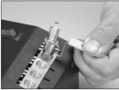
6.16 Remove the connector holder from the oven.
