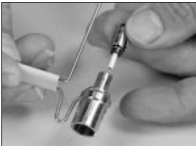
3.4 Load the connector onto the ST* connector holder.
