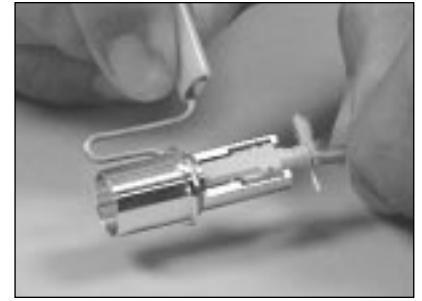
6.18 Push the cable until it stops against the connector. The aramid yarn should flare out over the backbone.
