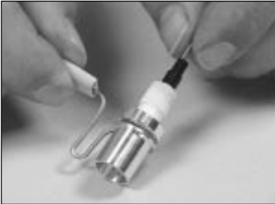
7.13 Slide the crimp ring over the backbone until it is against the connector.
