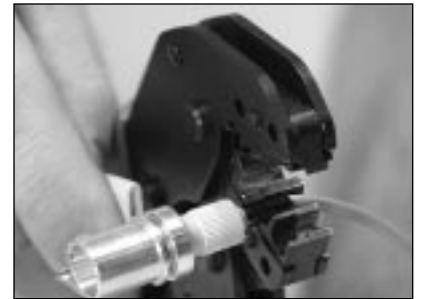
8.21 Crimp the smaller part of the crimp ring using the .137 cavity. (Use the .120 cavity for the optional 2.4 mm crimp ring)
