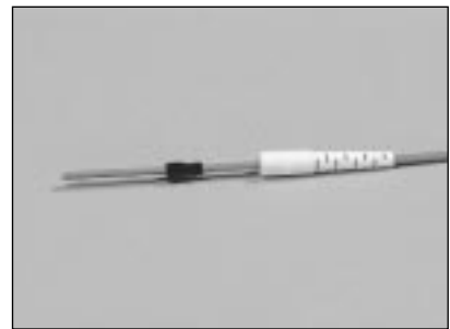
8.6 Place the strain relief boot and crimp ring on the cable.
