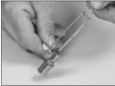
4.20 Secure the cable to the cable holder.
