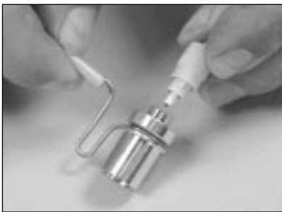
8.4 Load the connector into the FC connector holder. Align the key on the connector with the key way on the connector holder.
