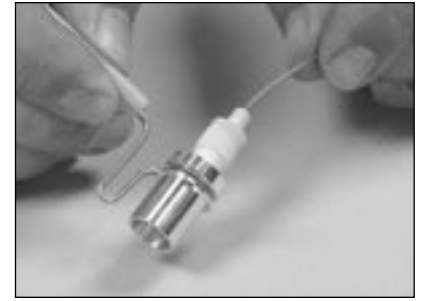
7.12 Push the fiber until it stops.
