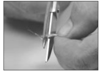
6.15 Cut the aramid yarn to \frac{5}{16} " (8 mm) long.
