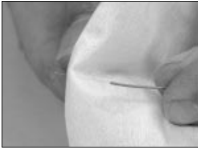
5.10 Clean the fiber with a lint free cloth moistened with isopropyl alcohol.
