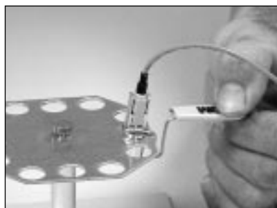
6.23 Place the connector holder into the cooling stand. The cooling time is about 3 minutes.
