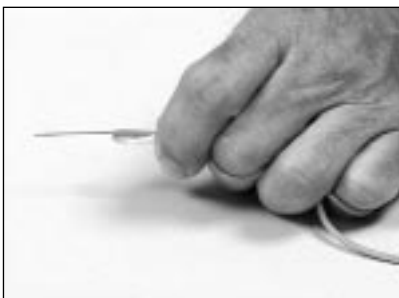
8.10 To prevent the buffered fiber from being pulled out, lace the cable through your fingers.
