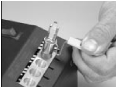
5.11 Remove the connector holder from the oven.
