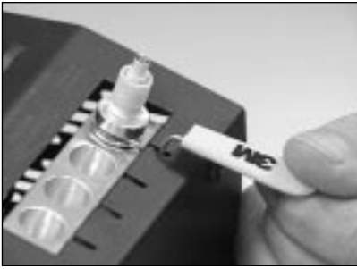
7.10 Remove the connector holder from the oven.
