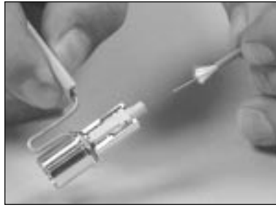
6.17 Gently insert the fiber into the connector.
