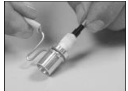
8.18 Slide the crimp ring over the aramid yarn until it is seated against the connector.
