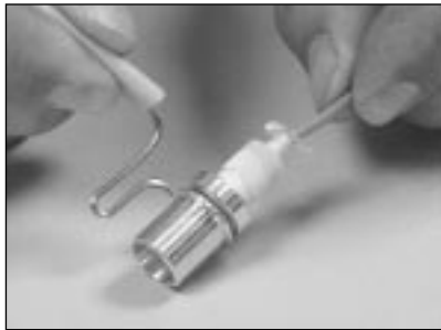
8.17 Push the cable until it stops against the connector. The aramid yarn should flare out over the backbone.
