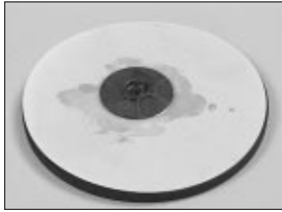
11.20 Place the jig on the lapping film.
