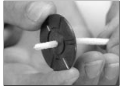
11.9 The second possibility is that the hole in the jig may have adhesive in it. Saturate a pipe cleaner with isopropyl alcohol and move it back and forth in the jig to remove the adhesive.
