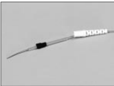
5.7 Place the strain relief boot, clear strain relief tubing and crimp ring on the fiber.
