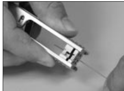
3.8 Remove the buffer in small pieces until \frac{5}{8} "– \frac{3}{4} " (16–19 mm) of the buffer has been stripped.
