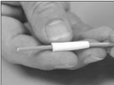
4.7 Place the strain relief boot on the cable.
