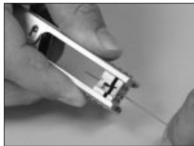
5.8 Remove the buffer in small pieces until \frac{1}{16} "– \frac{5}{8} " (14-16 mm) of buffer has been stripped.
