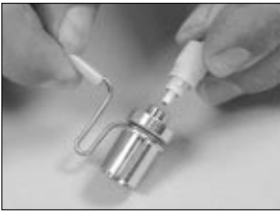
7.4 Load the connector into the FC connector holder. Align the key on the connector with the key way on the connector holder.
